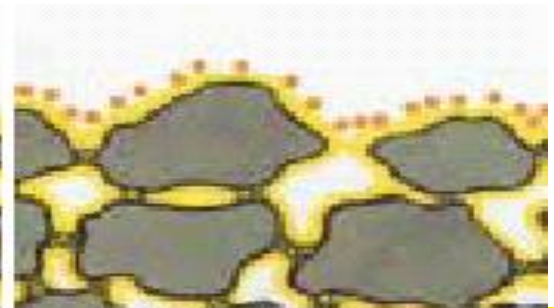
Improve early life skid resistance by sanding
